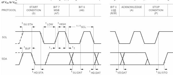
*l*<sup>2</sup>C-bus timing diagram.
