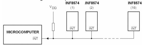
Application of multiple INF8574s with interrupt.
